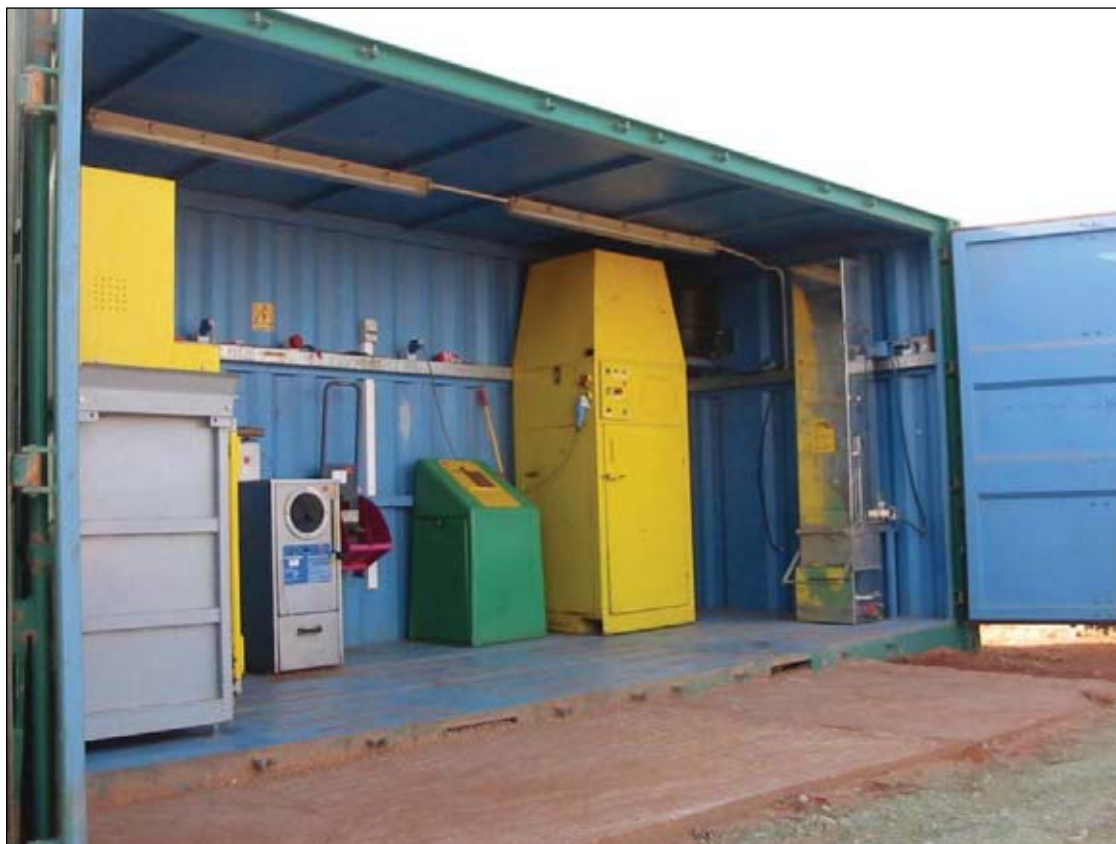
A patented Mobile Materials Recycling Facility is an easily transported container that houses all equipment needed to process waste at a project site. An integral generator and a combined office-store are supplied in a second unit not shown.
